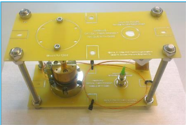
Figure 1: PCB Transport tool for CRM1-COE
