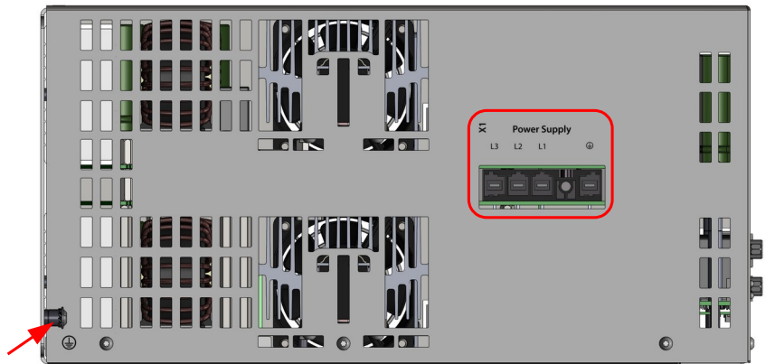
Figure 7: AC-power supply connector (X1) TSP700-40
