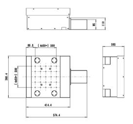
\*Interface dimensions from MZH400 in the middle of vertical stroke
