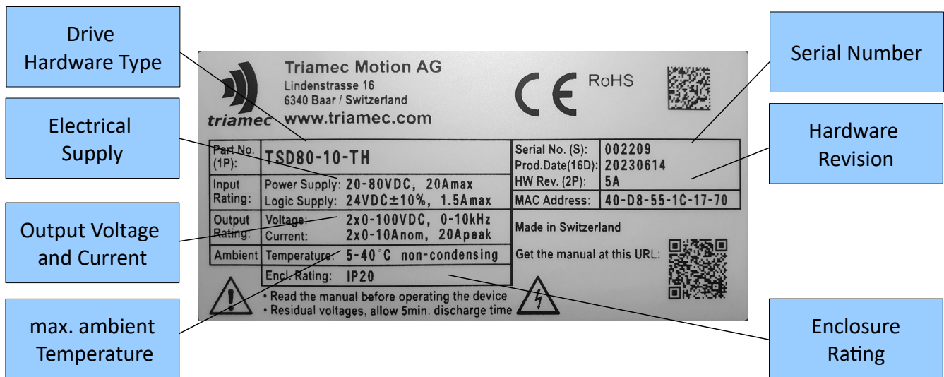
Figure 1: Nameplate of the TSD series servo drives
